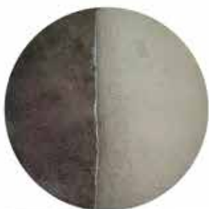
CMR 257 Ceramic Gray Casting Slip Total Shrinkage 6 %
