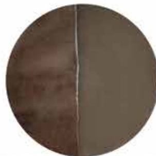
CMR 252 Ceramic Brown Casting Slip Total Shrinkage 6 %
